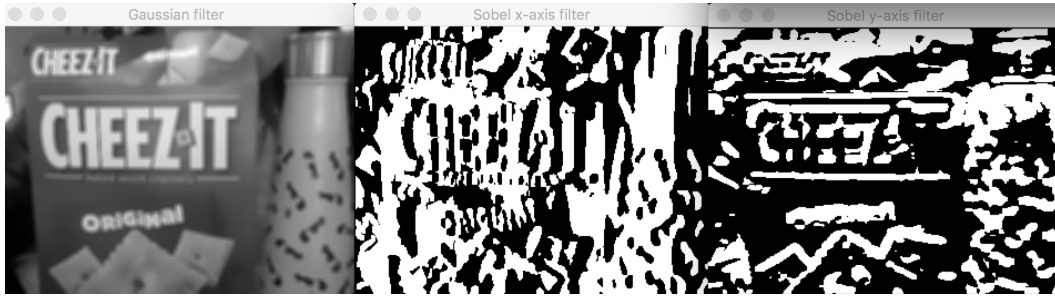
Figure 1: The first steps of the Canny Edge algorithm in OpenCV
